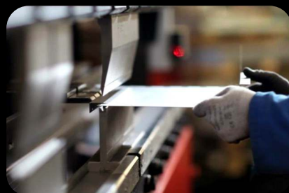
SHEET METAL BENDING
